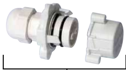
7. Quick Connect Plug Kit. This innovative plug kit is supplied with a range of colour-coded cable seals, allowing it to be connected to a range of cable thicknesses. It simply plugs into the rear of the QC LED Light and is secured with three screws. P/N LED375
